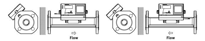
NB: For meters □DN100 MULTICAL® or the PULSE TRANSMITTER **cannot** be fitted directly on the flow part.
