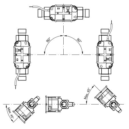
${\tt ULTRAFLOW}^{\scriptsize @}$  54 may be installed horizontally, vertically or at an angle.
