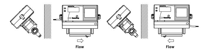
Glands and short direct sensor fitted in ULTRAFLOW® 54 ( $G^{3}/_{4}$  ( $R^{1}/_{2}$ ) and G1 ( $R^{3}/_{4}$ ) only).
