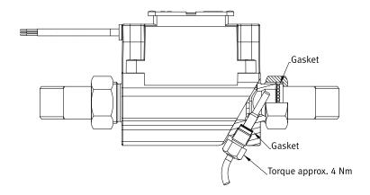
Flange meter with MULTICAL®/PULSE TRANSMITTER fitted directly on ULTRAFLOW® 54.
